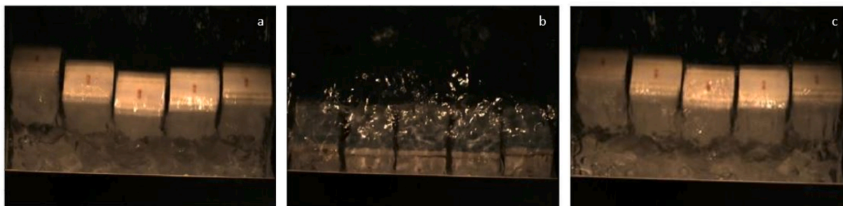
Fig. 8. a) Presence of transverse waves, b) Flow separation and turbulence, c) Vortex shedding.
