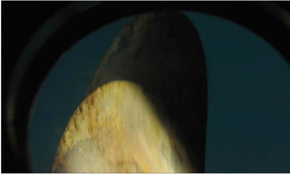
Fig. 6. Full-scale trial cavitation observation – 600 engine rpm.
