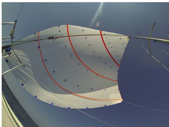
Fig. 4. Picture of the flying spinnaker from the camera located on the foredeck looking upward. Left: raw image with barrel effect due to the wide angle lens; right: same image after correction determined by the calibration process. Note the straight forestay which appears curved in the raw image.
