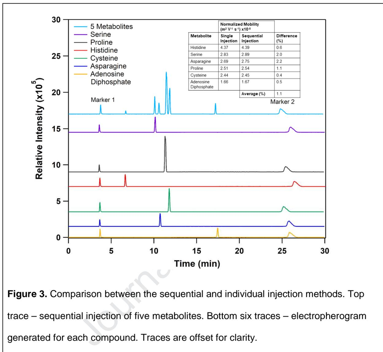
**Figure 3.** Comparison between the sequential and individual injection methods. Top trace – sequential injection of five metabolites. Bottom six traces – electropherogram generated for each compound. Traces are offset for clarity.
