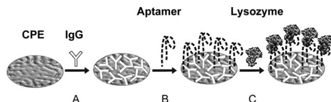
**Scheme 1.** Preparation steps of an anti-lysozyme aptasensor: (A) carbon paste electrode (CPE)-blocking step, (B) aptamer immobilization, and (C) lysozyme binding event.
