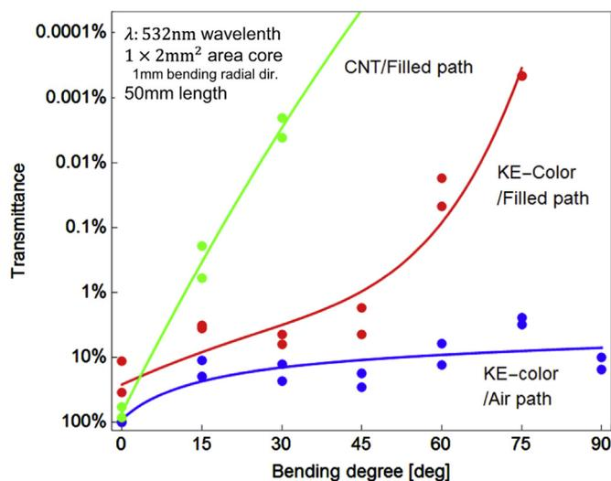
**Fig. 4.** Experimental transmittance of the flexible black-PDMS/PDMS light channel as a function of the bending angle. Blue indicates air channel (hole) in CB:PDMS cover, red indicates PDMS channel covered with CB:PDMS, and green indicates PDMS channel covered with CNT:PDMS. (For interpretation of the references to color in this figure legend, the reader is referred to the web version of this article.)
