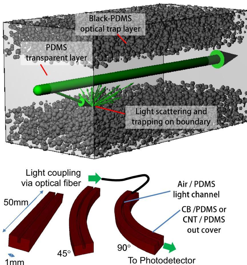
**Fig. 3.** Schematics of a PDMS/black-PDMS light channel and light propagation between the boundary structures (top) and schematics of bent light channels without covering black-PDMS for the trapping investigation (bottom).
