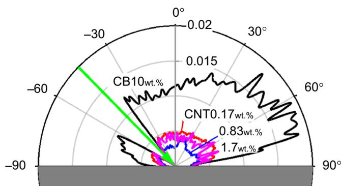
**Fig. 5.** Polar-plotted scattering intensity from the boundary of PDMS/black-PDMS. Black line indicates CB:PDMS of carbon black concentration of 10 wt%, magenta, blue and red lines indicate CNT:PDMS of carbon nano tube concentration of 1.7, 0.83 and 0.17 wt%, respectively. (For interpretation of the references to color in this figure legend, the reader is referred to the web version of this article.)
