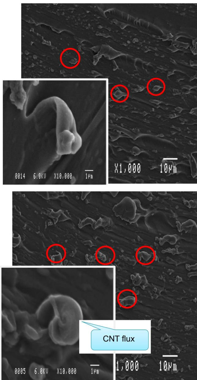
**Fig. 6.** Scanning Electronic Microscope image of the cut-surface of the black-PDMS. Above image is from CB:PDMS of carbon black concentration of 10 wt%, and below image is from CNT:PDMS of carbon nano tube concentration of 0.19 wt%. Red circles indicate the aggregated black particle due to the high concentration diffusing. (For interpretation of the references to color in this figure legend, the reader is referred to the web version of this article.)
