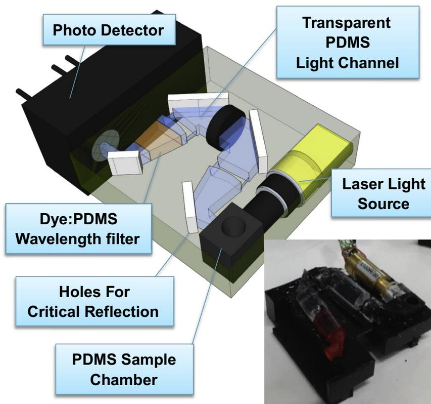
**Fig. 1.** Schematic of PDMS/Carbon-PDMS module for laser induced fluorescence detection. All optical component is covered black-PDMS molding. Right bottom image is the photo image of the assembled components for the pumping at 532 nm and measuring at 600 nm without covering black-PDMS.
