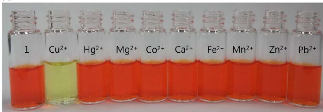
Figure 2. (a) Emission spectrum of chemosensor 1 ( 3.0 \times 10^{-5} M) obtained in PBS buffer (DMSO:H 2 O = 1:9, v/v, pH = 7.3) upon titrated with Cu 2+ , Hg 2+ , Mg 2+ , Co 2+ , Ca 2+ , Fe 2+ , Mn 2+ , Zn 2+ , and Pb 2+ . Excitation wavelength is 400 nm. Emission wavelength is 567 nm. (b) The Emission intensity enhanced index ( F/F_0 ) in the presence of 4 equiv. of various metal ions.
