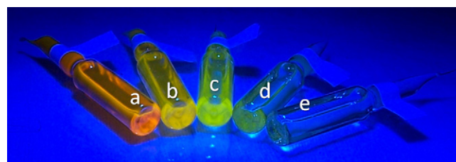
Fig. 6. PL images of \text{N}_2 enriched solutions (50 \mu\text{g/ml} ) exposed to the commercial phototherapy system from (a) 0 min, (b) 60 min, (c) 120 min, (d) 180 min and (e) 240 min.
