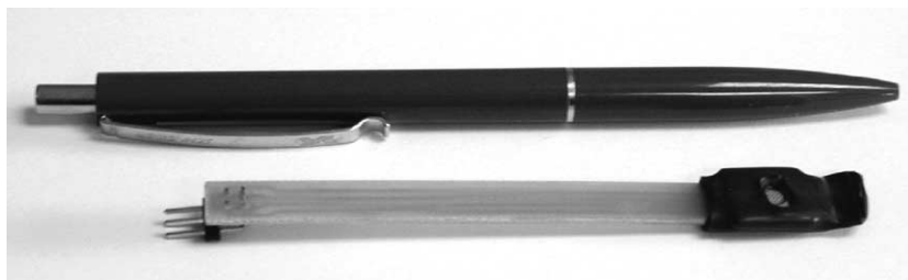
Fig. 4. Photo of the hydrogel-based sensor.
