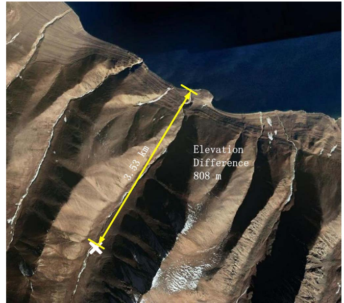
Fig. 9. A typical selection result of linking an existing lake and a newly built upper reservoir. The cross is the specific site selection for a scheme of upper reservoir. The latitude and longitude coordinates of the cross are, respectively. The elevation of the cross is 5348 m. The elevation of the lake is 4540 m. The figure was created from Google Earth.
