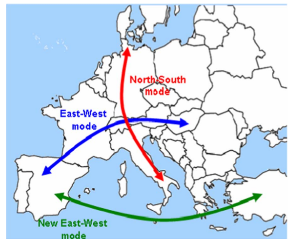
Fig. 9. Dominant inter-area modes in the ENTSO-E system.
