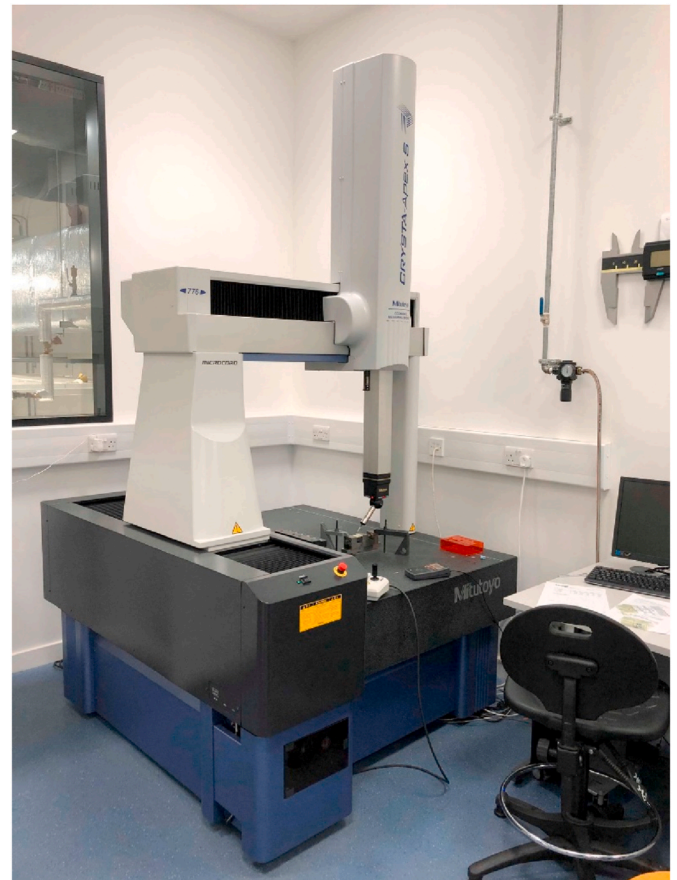
Fig. 7. Stylus profilometer: Mitutoyo Crysta Apex S, utilises a stylus of radius 0.3 mm to measure flat surfaces with a resolution of 0.1 \mu\text{m} [30,67].
