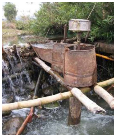
Fig. 6. Standing Pico-Hydro Unit in Khaiveng Village, Kham District, Xieng Khouang Province. (Used with permission of M Smits [27]).
