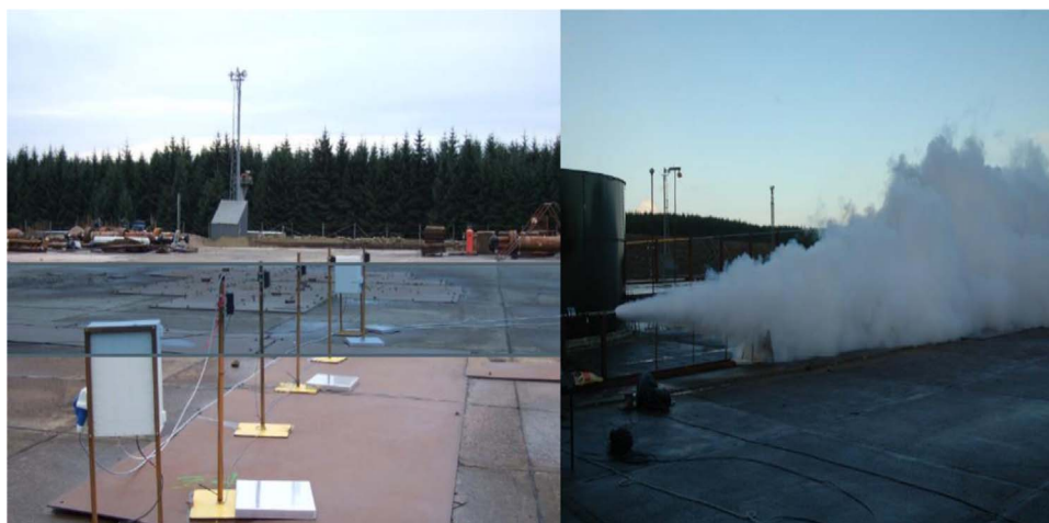
Fig. 14. Photographs of the instrumented target and of a release of CO 2 through a 0.5 in. orifice [142].
