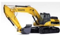
Excavator Engine Power Range: 60 – 400 kW
