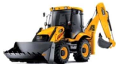
Backhoe Loader Engine Power Range: 50 - 100 kW
