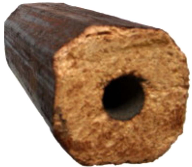
Fig. 13. Briquette with a concentric hole produced from a screw extruder/press. Used with permission by New-Air Technical Services Ltd. Leicester, England from [27].
