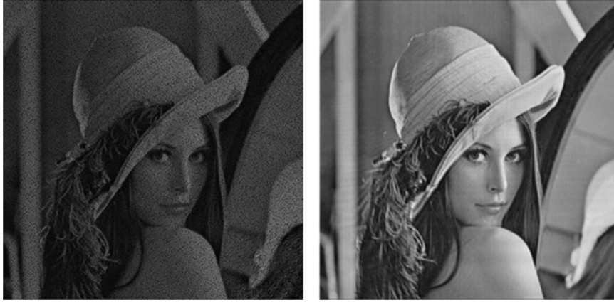
Fig. 9. Reconstructed images at five iterations. With random phase (left). With the proposed method (right).
