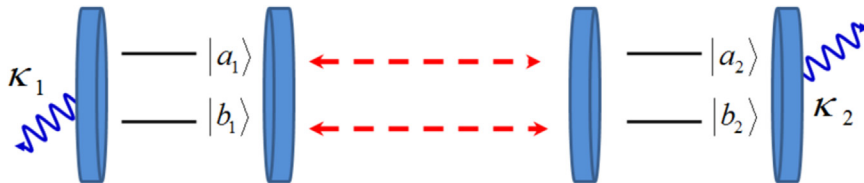
Fig. 1. Two two-level atoms, initially prepared in an entangled state, trapped in two cavities having structured vacuum reservoir surrounded by vacuum environment.
