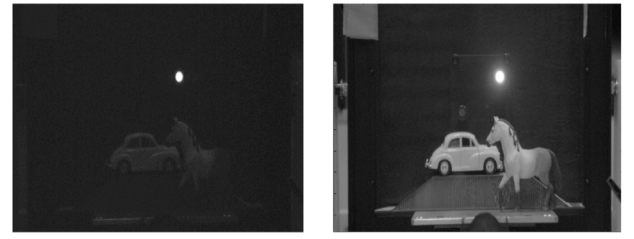
Fig. 9. Hybrid calibrated-natural 78 dB test scene images captured for the proposed minimal images multi-exposure method for HDR image recovery. Exposure times: Left image: 59 \mu\text{s} and Right Image: 5.9 \text{ ms} .
