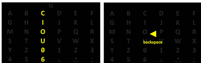
Fig. 1. User display for the P300 Speller BCI. Left: intensification of a column of the matrix display. Right: feedback moment (the identified symbol is displayed on the screen).
