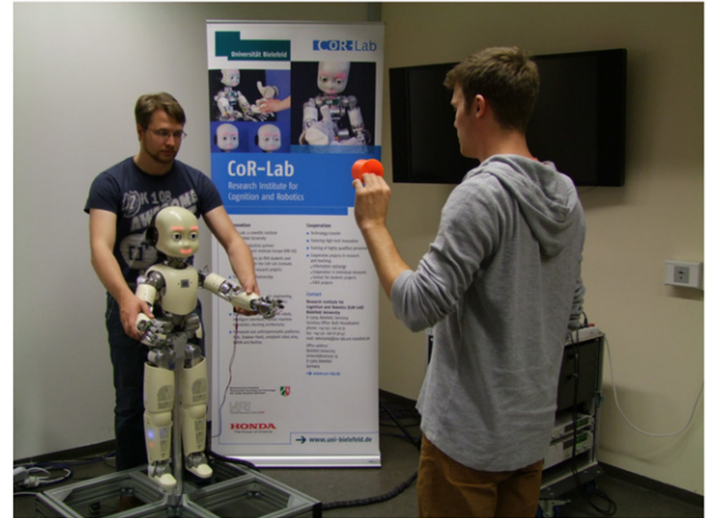
Fig. 6. Kinesthetic teaching of the humanoid robot iCub. One tutor guides iCub's left arm and another holds a red cup to point at in his left hand. (For interpretation of the references to color in this figure caption, the reader is referred to the web version of this article.)
