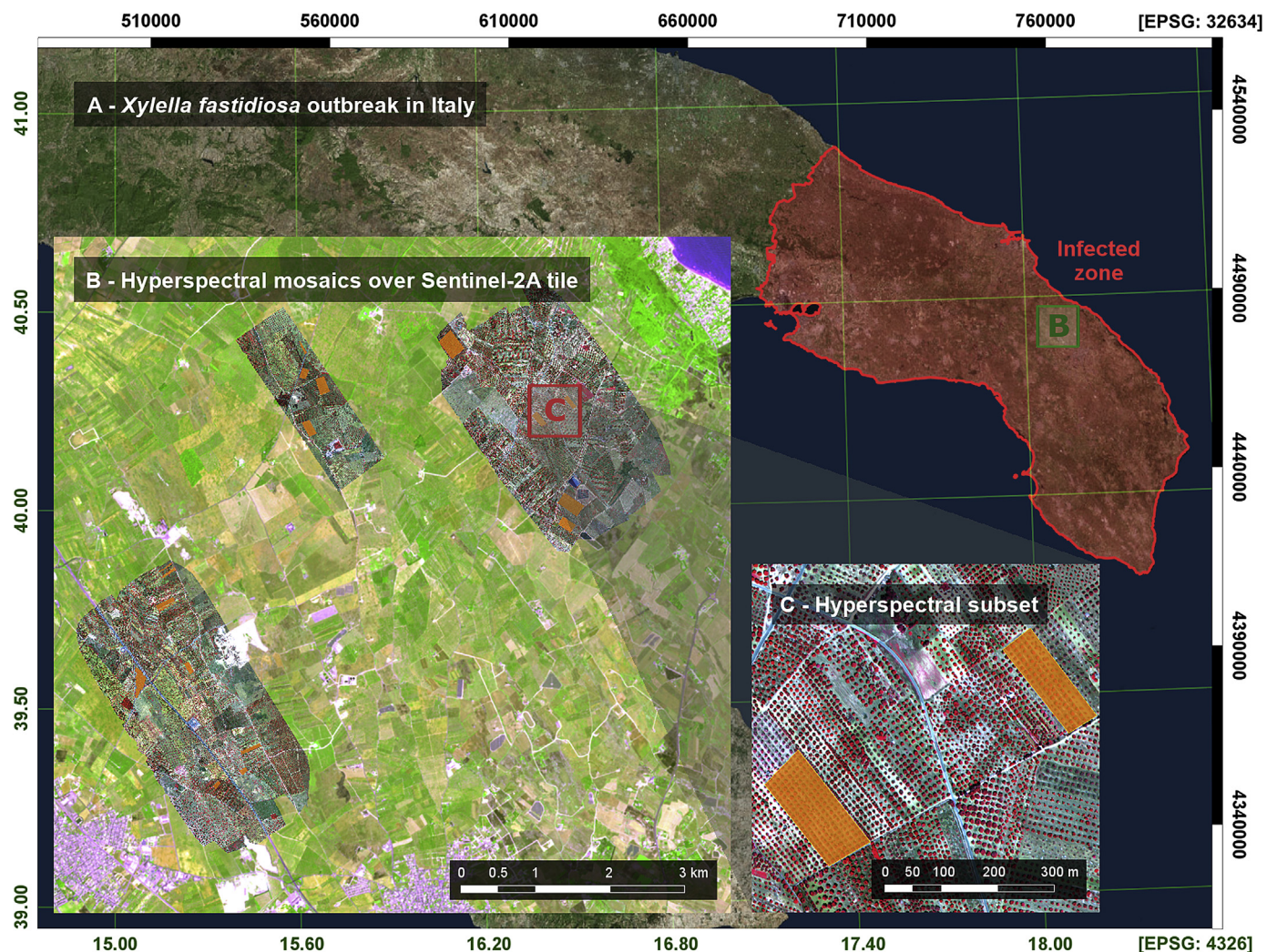
Fig. 1. Sentinel 2A scene of southern Italy (large inset, A) with an overlay (green box, B) in which airborne hyperspectral mosaics are shown. The three hyperspectral images were acquired from aircraft on 28 June 2016 with a micro-hyperspectral imager (red box, C) yielding 40-cm spatial resolution. The infected zone highlighted in the main map (A) outlines the area where Xylella fastidiosa has been observed as of March 2018 (Commission Implementing Decision (EU) 2018/927, 2018). (For interpretation of the references to colour in this figure legend, the reader is referred to the Web version of this article.)
