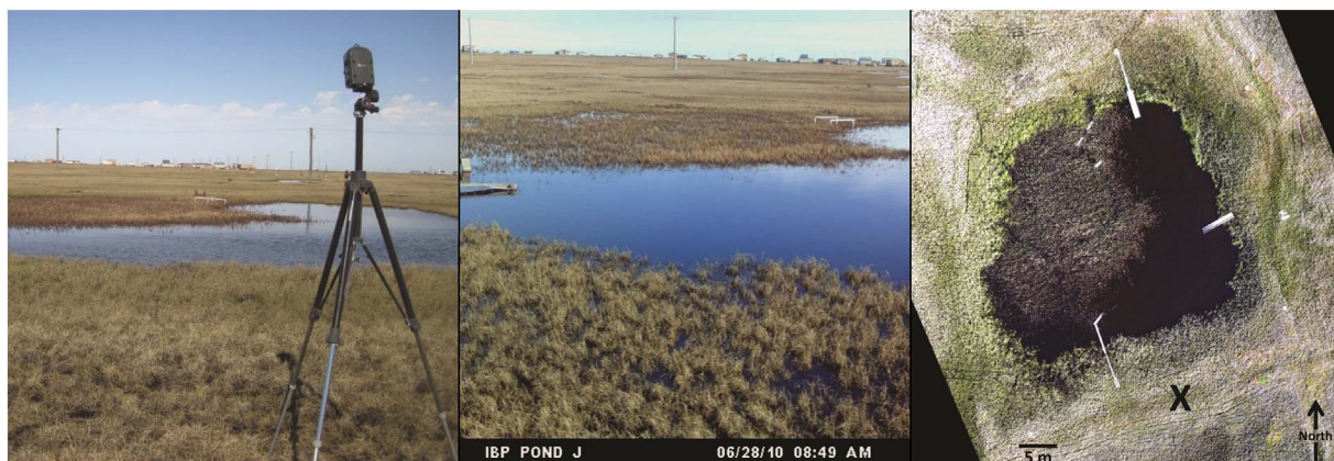
Fig. 1. (Left) Near-surface, oblique camera mounted on a tripod facing north at IBP Pond J, (middle) a sample photo taken from this system and (right) a kite aerial photograph of the site where camera location is marked with an X.
