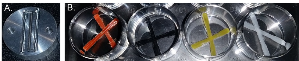
Fig. 5. A) aluminum dog bone injection mold used during the current study, B) successfully injection molded PCL samples 5–8 (from left to right); Doxorubicin, MWCNT, Ferrocene, and pure PCL.
