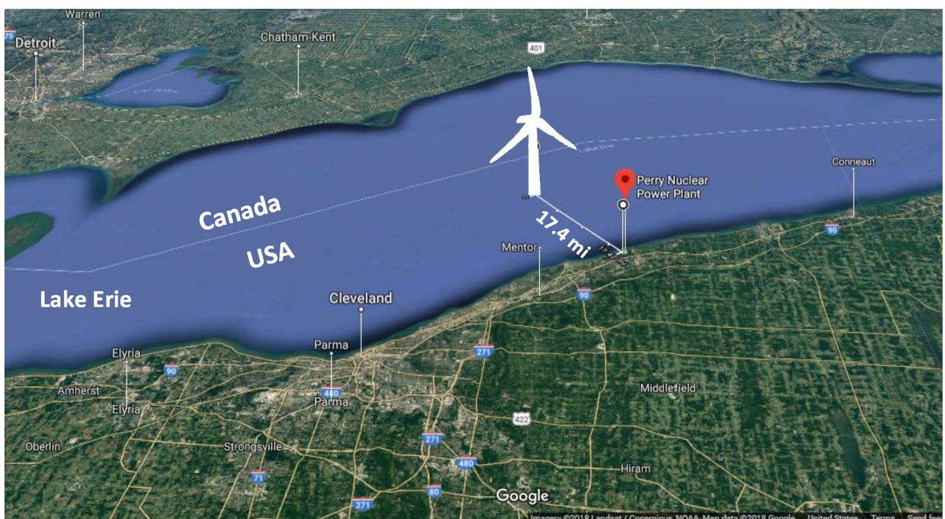
Fig. 2. Map of location of the considered 1000 MW offshore wind power plant, 17.4 miles off the shore of Lake Erie in Perry, Ohio.
