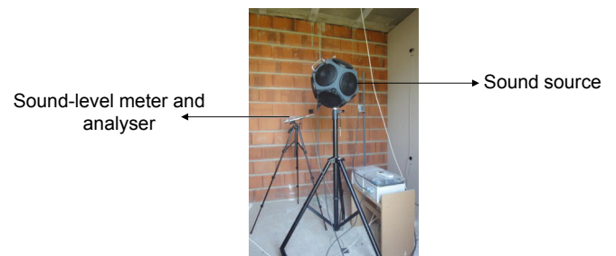
Fig. 6. Equipment used to perform the acoustic measurements in situ .
