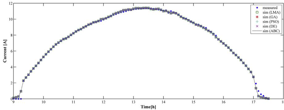
**Fig. 3.** Evolution of the DC-current of the PV system 1 using SAPM for clear sky day (December 09th, 2013).
