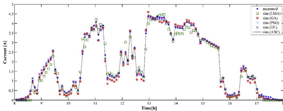
Fig. 8. Evolution of the DC-current of the PV system 3 using 5PM for cloudy day (November 12th, 2012).
