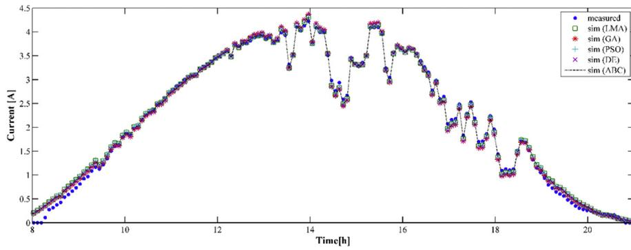
Fig. 5. Evolution of the DC-current of the PV system 2 using SAPM for semi-cloudy day (May 12th, 2012).
