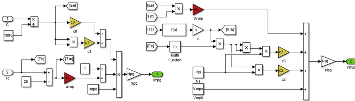
Fig. 2. Simulink block diagram for the SAPM.
