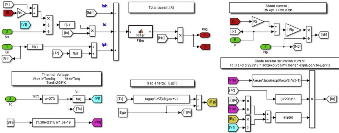
Fig. 1. Simulink block diagram for the 5PM.
