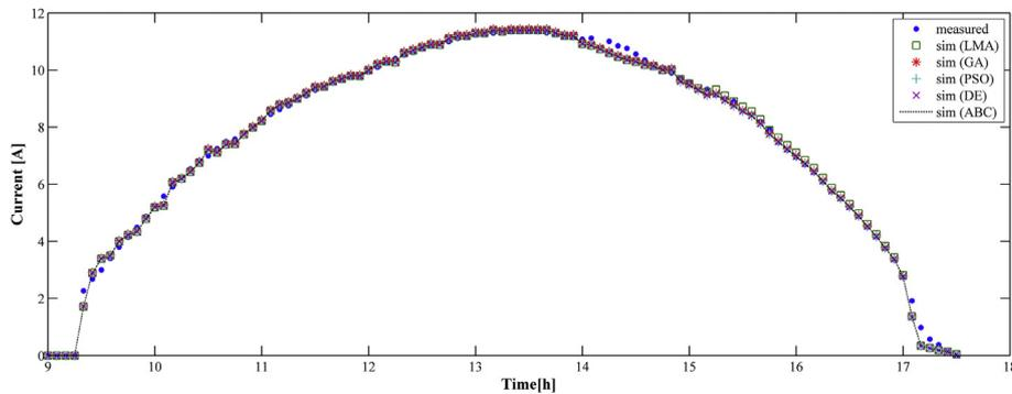
**Fig. 4.** Evolution of the DC-current of the PV system 1 using 5PM for clear sky day (December 09th, 2013).
