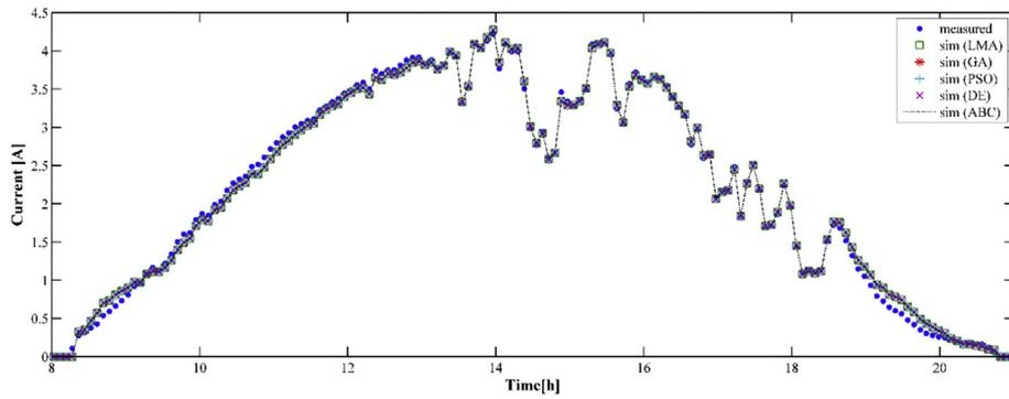
Fig. 6. Evolution of the DC-current of the PV system 2 using 5PM for semi-cloudy day (May 12th, 2012).
