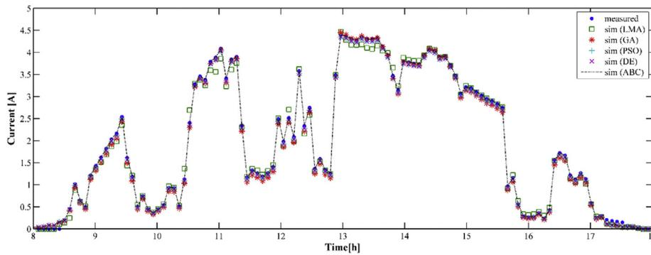
Fig. 7. Evolution of the DC-current of the PV system 3 using SAPM for cloudy day (November 12th, 2012).
