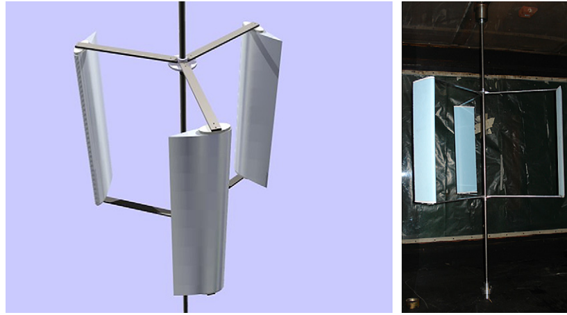
Fig. 1. CAD model of the turbine model assembly and the model turbine in the wind tunnel.
