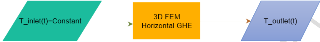
Fig. 3. Flow chart for the short-term performance of horizontal GCHP model
