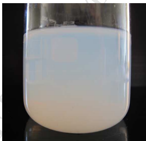
Fig. 2. The prepared nanofluid with 0.6% vol. after two months
