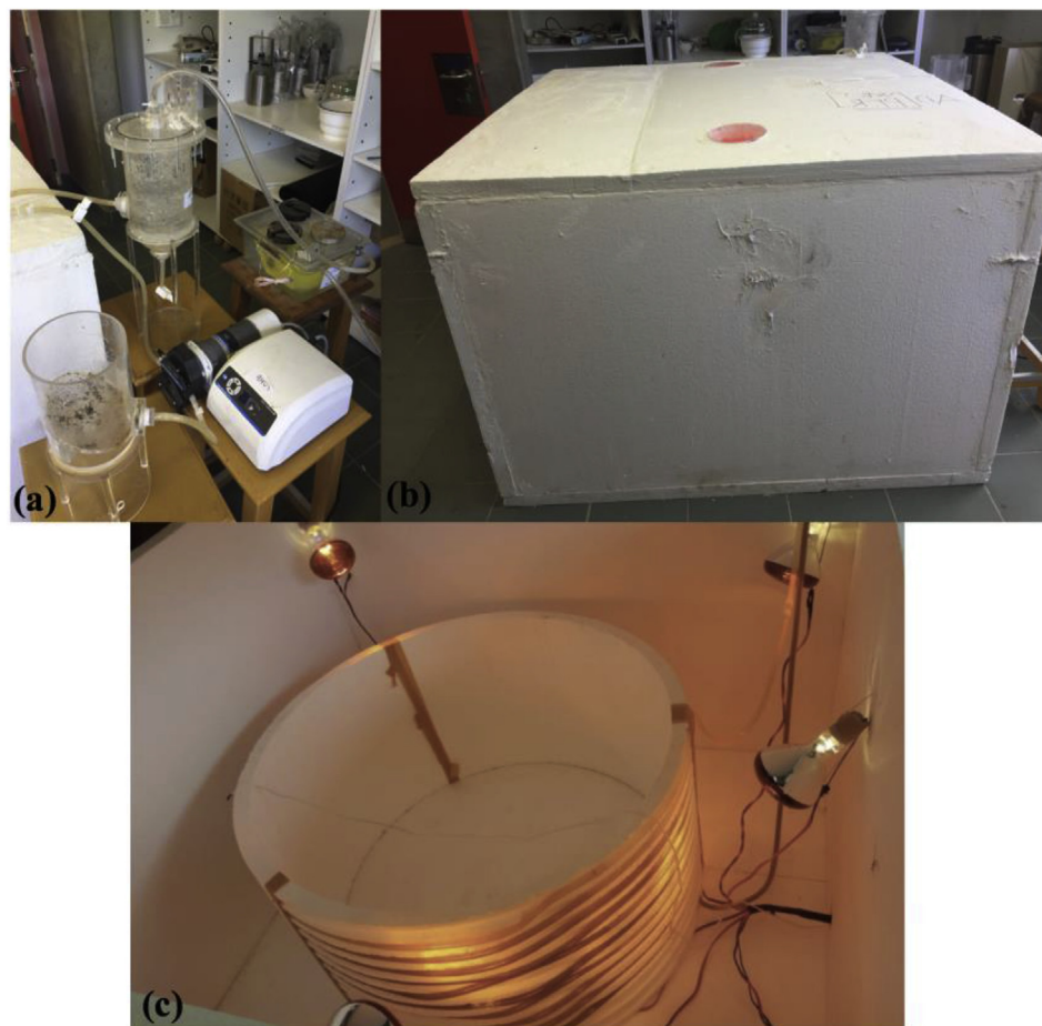
Fig. 2. Experimental Setup: (a) Feeding tank, peristaltic tank, and digestate tank; (b) constant temperature chamber; (c) FSAD tube, coiled around a Styrofoam cylinder.
