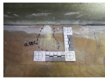
(b) Day 28: Further channel cracking arising on
