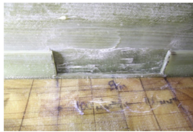
(a) Day 7- Day 9: Defect induced into the internal surface of the blade at a blade-web boundary
