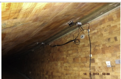
(b) AE sensors mounted the trailing edge side
