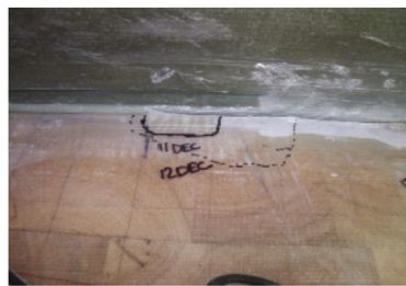
(a) Day 27: The start of damage propagation
