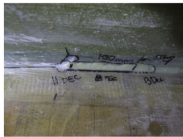
(c) Day 29: Delamination reached 0.15 m
