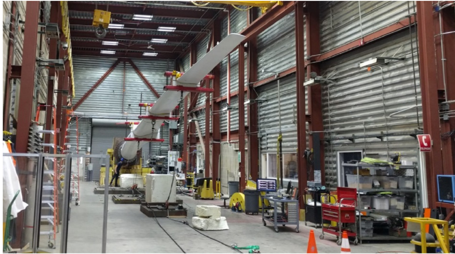
Fig. 10. Fabricated SUMR-D blade during static test.
