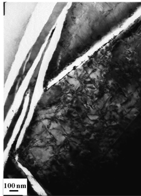
Fig. 2. TEM micrograph detailing dislocation debris the microstructure obtained at 250^\circ\text{C} .
