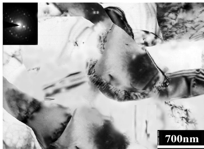
Fig. 12. Bright field TEM image of pure Al sample after 8 pass of the ECAP.
