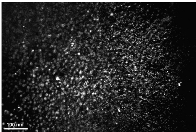
Fig. 9. Deformation microstructure after 40 cycles: three-part distribution in precipitate size.
