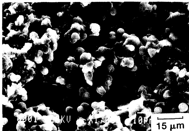
Fig. 7. Micrograph of the fracture surface of a porous carbon preform.
