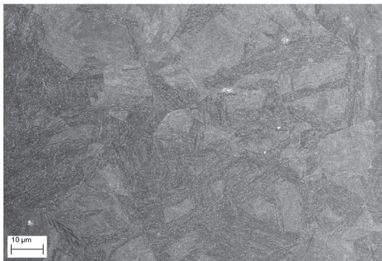
(c) Bainitic-martensitic microstructure of sample BM-3. Brighter areas are martensite, darker areas with dot pattern correspond to bainite, similar to sample FB-1 the white dots correspond to cementite.
