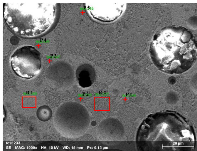
Fig. 3. Selected regions in the syntactic foam matrix microstructure for EDS analysis.
