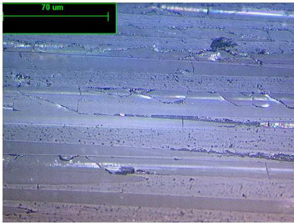
Fig. 12. Optical micrograph showing cracks in the glass fibres at 45° (see arrows) with respect to the fibre axis in second glass layer within GLARE after 50J impact on the substrate.
