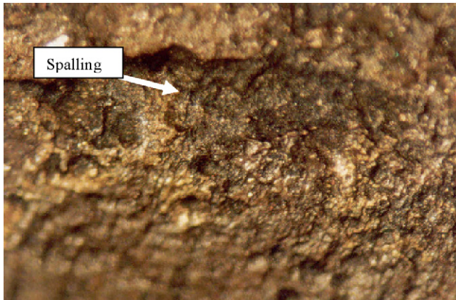
Fig. 8. Stereomicrograph of the low alloy steel containing 0.76% Cr (specimen 6) (70 \times ).
