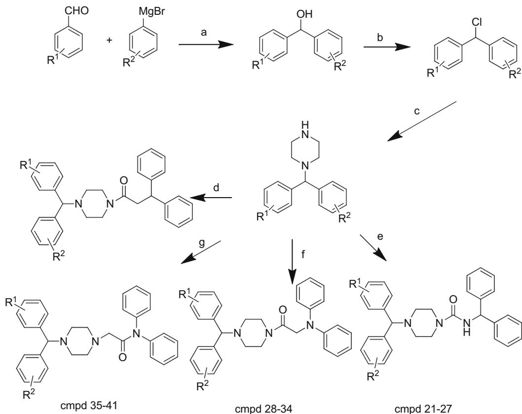
**Scheme 1.** Reagents and conditions: (a) ether, reflux; (b)  $\text{SOCl}_2$ , benzene, reflux; (c) anhydrous piperazine,  $\text{K}_2\text{CO}_3$ , KI,  $\text{CH}_3\text{CN}$ , reflux; (d) 3,3-diphenylpropanoic acid, EDC, DMAP, rt; (e) diphenylmethyl isocyanate, rt; (f) 2-(diphenylamino)acetic acid, EDC; (g) 2-bromo-*N,N*-diphenylacetamide,  $\text{NaHCO}_3$ ,  $\text{CH}_3\text{CN}$ , reflux.
