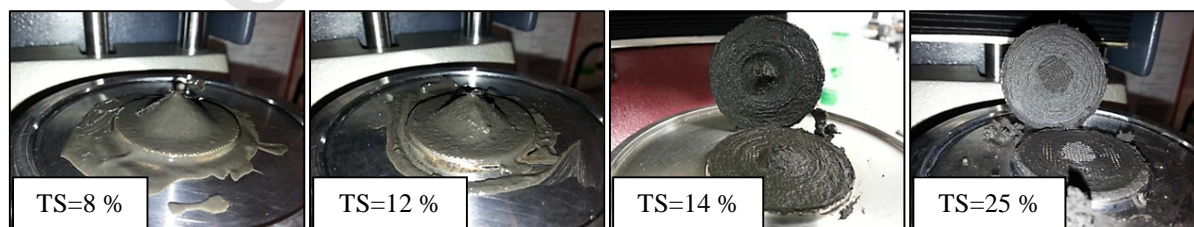
Figure 10 – Surface profile of sludge between parallel plates at the end of experiments.
