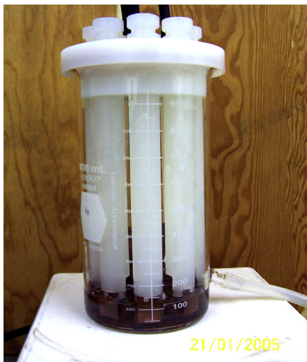
Fig. 1 – Modified CDC reactor showing the paired copper coupons (1.5 × 1.7 cm inside, 1.5 × 1.3 cm outside on the rods), base plate (bottom of the reactor) and the blade in the center.
