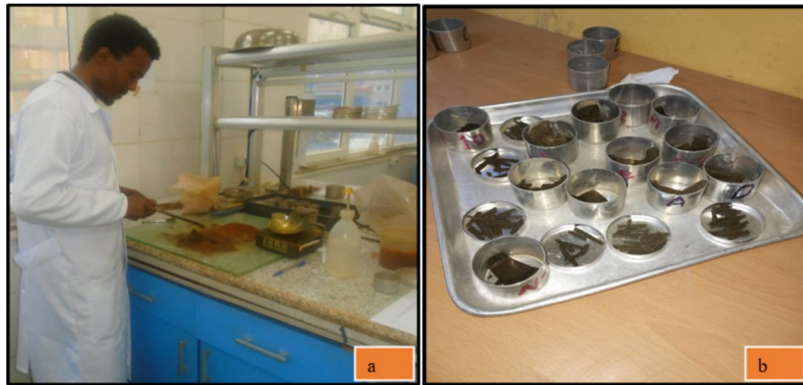
Fig. 5 Shows atterberg limit test preparation (a) and rolled sample for plastic limit test (b)
