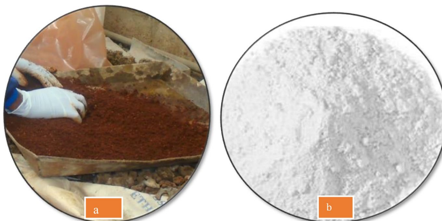
Fig. 3 Shows the prepared soil spacemen (a) and Quicklime powder (b) to be mixed
