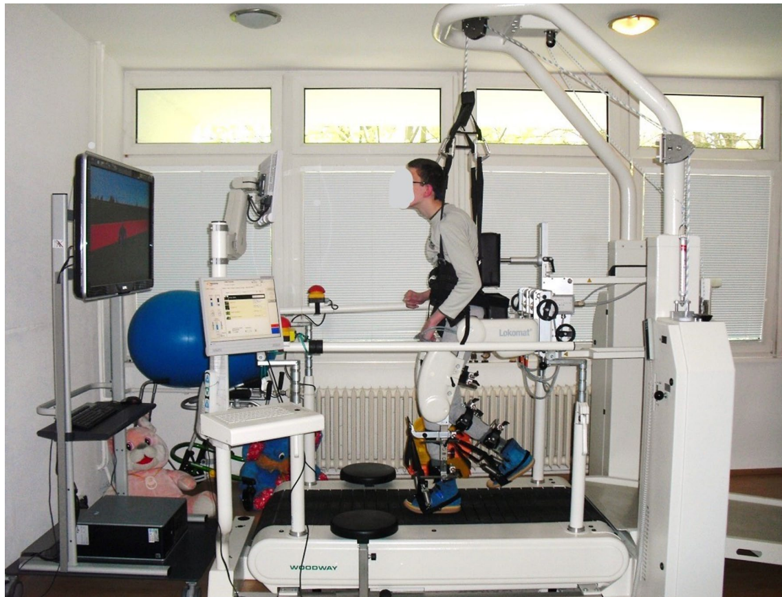
Fig. 2 Robot-assisted locomotion therapy in a virtual reality-based environment in the Lokomat®
