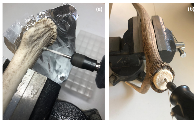
Figure 1 – Drilling procedure of Mesola red deer antler: (a) Weathered antler, held in a vice; the basal portion of the beam pulverized in a single hole to 8 mm depth from the seal and the powder is collected through tinfoil in a 2 ml safelock tube. The tinfoil funnel is open and the transparent side shield is not mounted on the drill to better show the drilling position; (b) Antler housed in a storehouse, held in a vice; the seal pulverized in a single hole in the middle of the antler base.
