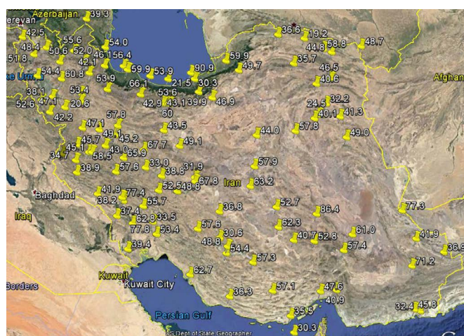
Figure 6: Estimated gust wind speed estimates based on reverse Weibull distribution at 109 meteorological stations of Iran.
