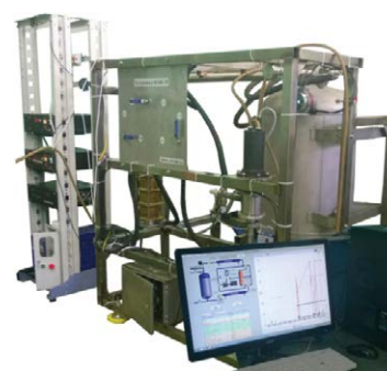
Figure 15: Ultrasonic Processing Facility I100-35 / 2 with magnetic reactor.
