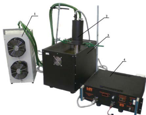
Figure 4: General view of experimental ultrasonic device IL10 - 4.0. 1. Unit of the autonomous cooling, 2. Ultrasound converter, 3. Generator, 4. Ultrasound bath.
