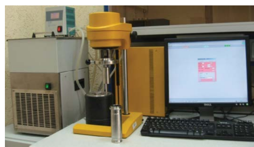
Figure 10: General view of the rotational viscometer Rheotest RN4.1.
