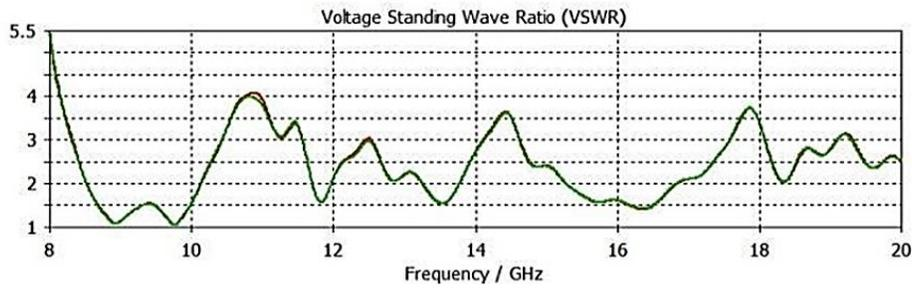
**Figure 5: Simulated VSWR vs. frequency characteristics of the antenna**
