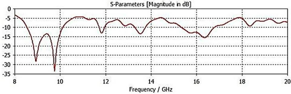
**Figure 4: Simulated reflection coefficient (S12) characteristics of antenna.**
