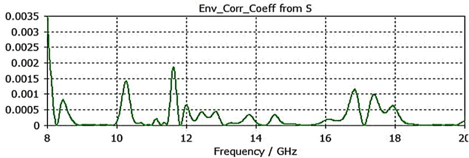
**Figure 6: Simulated ECC characteristics of the antenna.**
